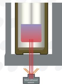
Mid-infrared wavelength light capable of penetrating the vessels
