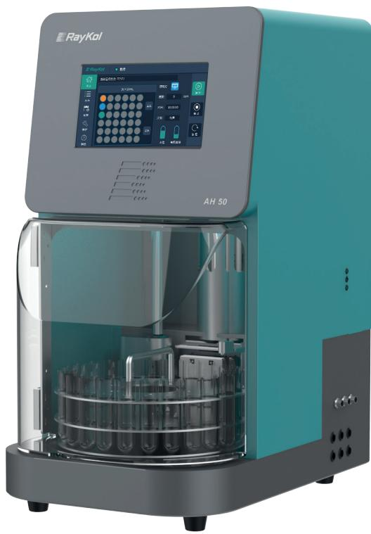
With the development of food safety and bio-medicine, automated homogenizers are more and more widely used in the sample pre-treatment of pesticide and veterinary drug residue detection to agricultural and livestock products, meat, eggs and milk. RayKol AH 50 is a versatile and high throughput automated homogenizer, it completely replaces manual process of adding solvent and homogenization. It can process up to 36 samples at one time, greatly improving the efficiency of sample pre-treatment.
