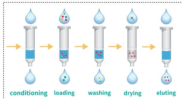
Solid phase extraction process is fully automated
