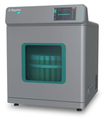
Microwave digestion utilizes the penetrability and activation reaction ability of microwave to heat the reagents and samples in the sealed container, so it can increase the pressure in the sample preparation container and the reaction temperature. Under microwave and sealed high temperature conditions, the samples can be quickly digested. The technology is mainly used for sample pretreatment of AAS, AFS, ICP, ICP-MS.
